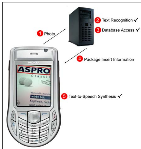
Figure 2: BaMoS System Architecture
