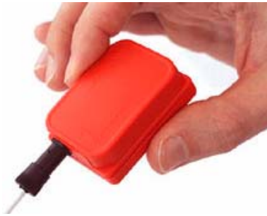
Figure 7: MTx inertial sensor.
